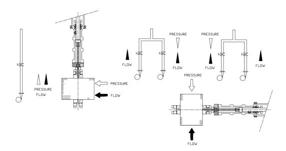
Special care should be taken to maintain the correct distance between the flanges and to ensure that they are parallel to the valve body. Incorrect alignment of the valve can cause deformations, which can lead to difficulties in operation.
