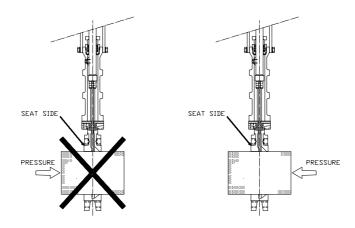
It should be noted that the direction of flow and differential pressure, do not always coincide.
